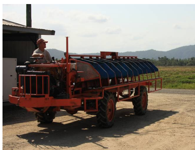
The banana harvester was modified to minimise soil compaction. Photo: DEEDI
